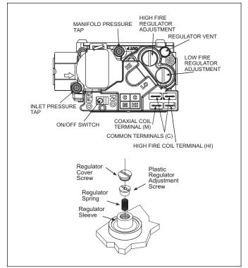
Figure 39 Gas valve and regulator adjustment
