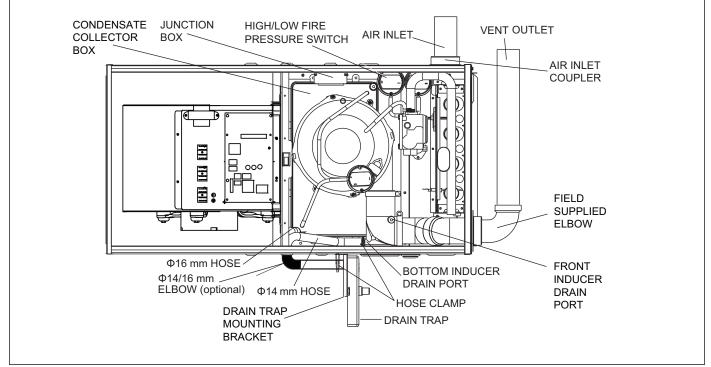
Figure 16 Horizontal Right-Hand Side Installation
