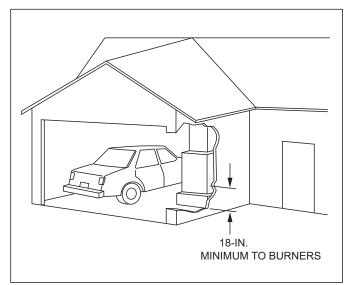
Figure 6 Installation in a garage
