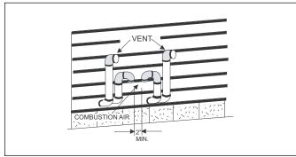
Figure 29 Double Horizontal Combustion Air Intake and Vent Termination
