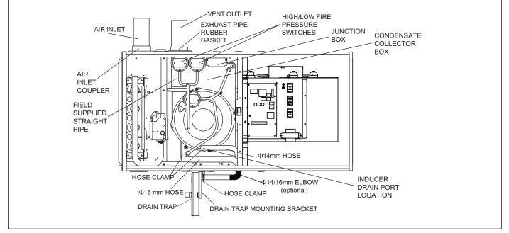
Figure 20 Horizontal Left Side Installation, Vent Through Side Panel
