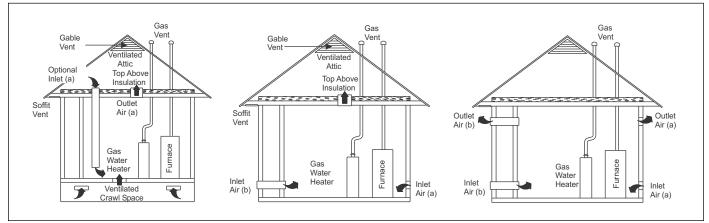
Figure 33 Ambient Combustion Air
