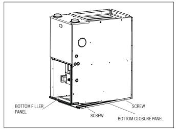
Figure 7 Removing bottom closure panel
