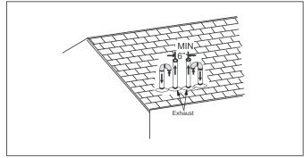
Figure 30 Double Vertical Combustion Air Intake and Vent Termination
