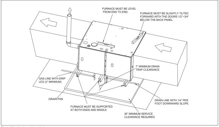
Figure 11 Horizontal Installation
