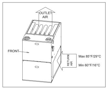
Figure 5 Return Air Temperature
