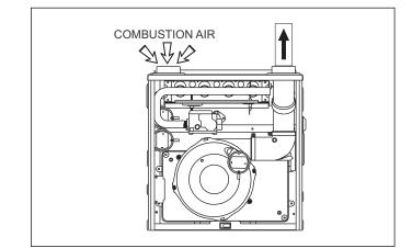
Figure 32 Combustion Airflow Path Through The Furnace Cabinet
