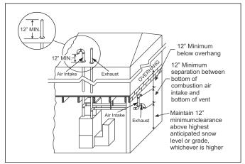
Figure 28 Termination Configuration - 2 Pipe Basement
