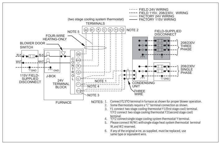
Figure 38 Heating and Cooling Application Wiring Diagram with 2-Stage Thermostat
