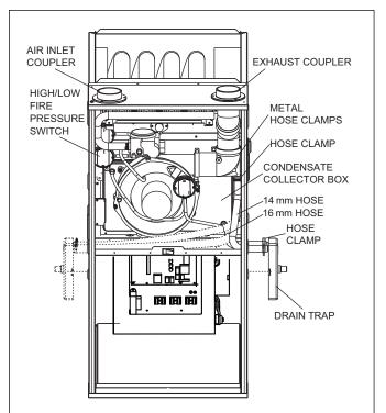
Figure 14 Upflow Installation, Top Venting
