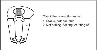
Figure 42 Burner Flame
