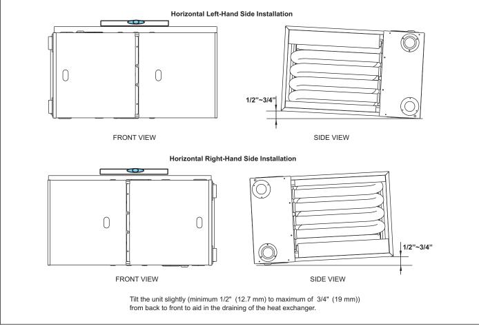
Figure 9 Horizontal Application-Setting Equipment
