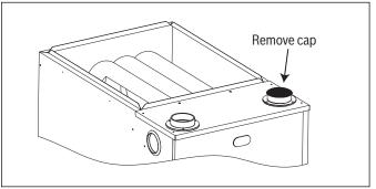
Figure 23 Protective Cap Removal
