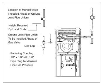
Figure 35 Typical Gas Pipe Arrangement
