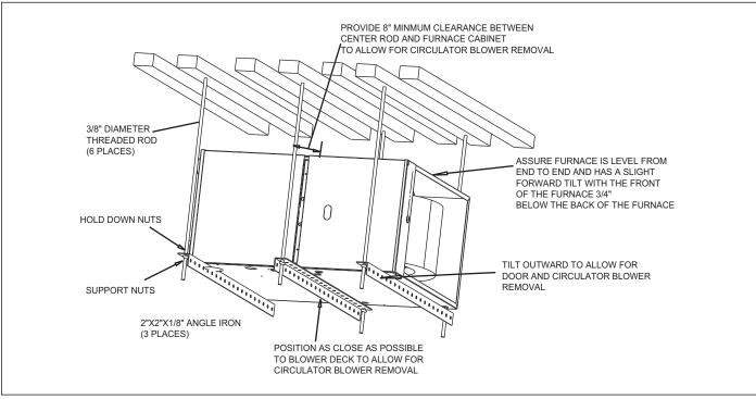
Figure 10 Horizontal Installation
