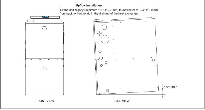
Figure 8 Upflow Application-Setting Equipment
