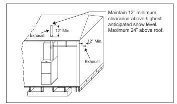
Figure 26 Termination Configuration - 1 Pipe, No
