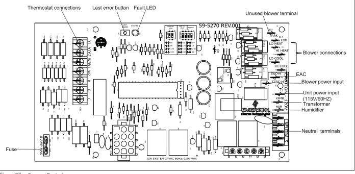
Figure 37 Furnace Control
