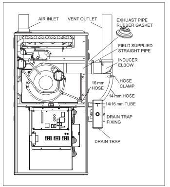
Figure 15 Upflow Installation, Right Side Venting
