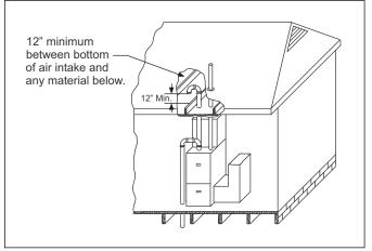
Figure 34 Attic and Crawl Space Combustion Air Termination
