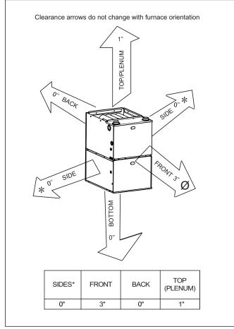
Figure 3 Minimum clearance from combustible construction
